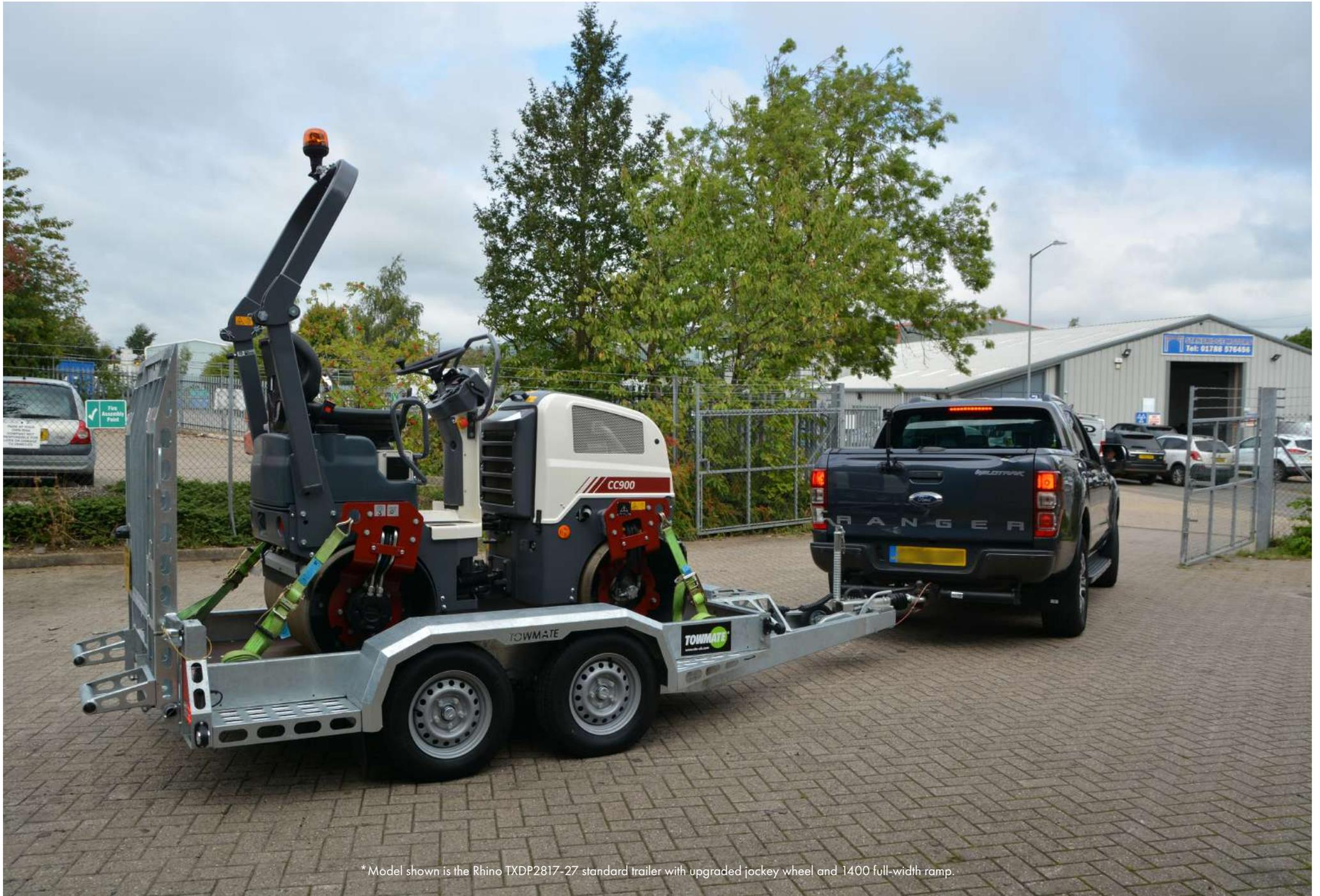
\* Model shown is the Rhino TXDP2817-27 standard trailer with upgraded jockey wheel and 1400 full-width ramp.
