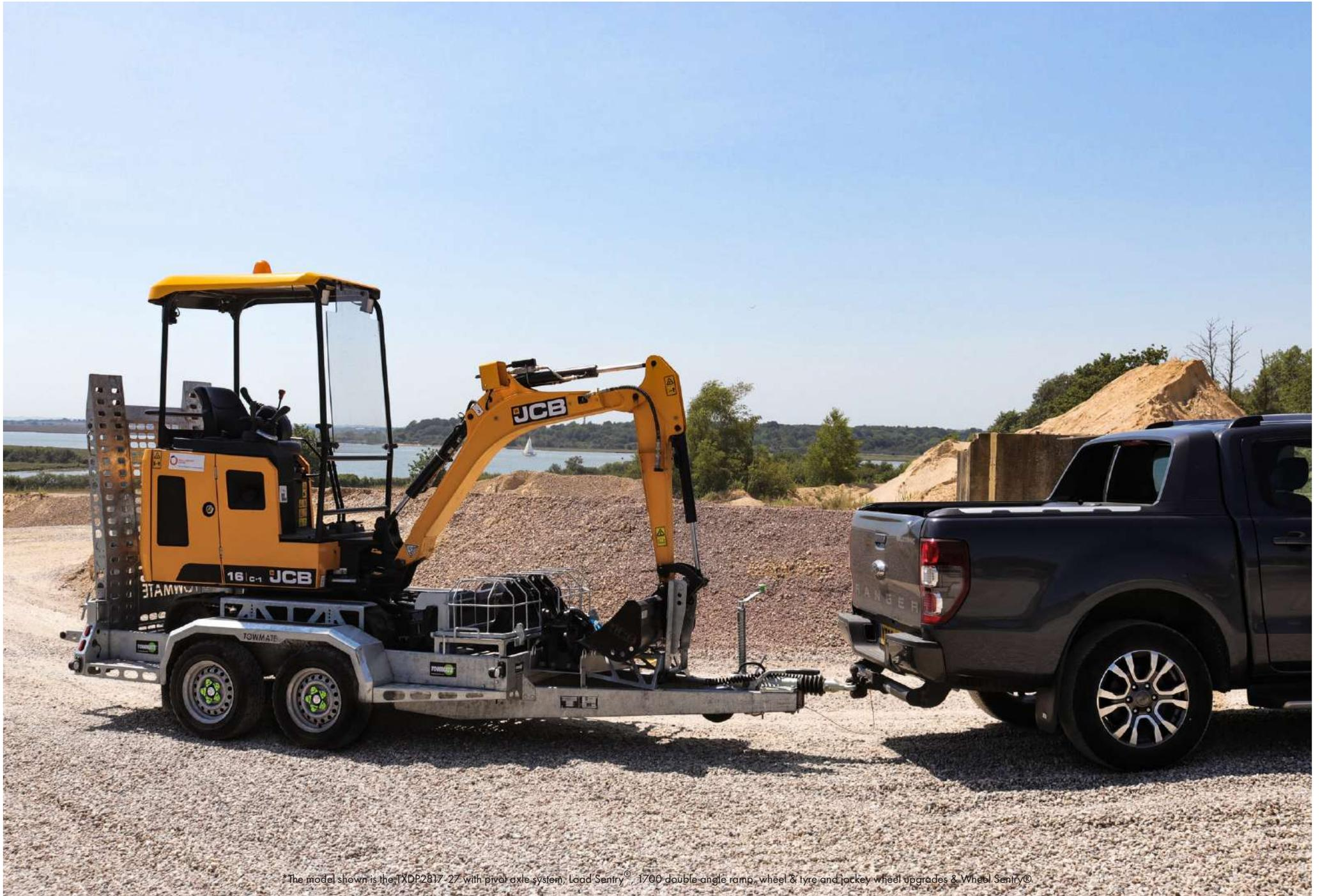
\*The model shown is the TXDP2817-27 with pivot axle system, Load Sentry<sup>®</sup>, 1700 double angle ramp, wheel & tyre and jockey wheel upgrades & Wheel Sentry<sup>®</sup>.
